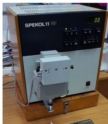
Fig. 6. Single-beam spectrophotometer with microprocessor „SPEKOL 11“.
