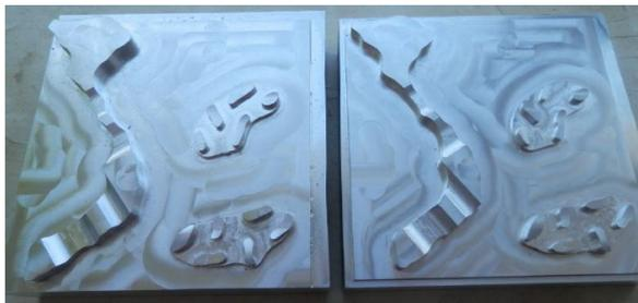
(a) detail 1 after finish milling by the variant without optimization (b) detail 2 after finish milling by the variant with optimization
