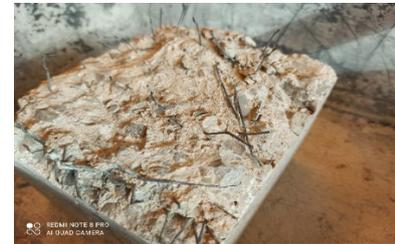
Fig. 2. Collecting of fibers.
