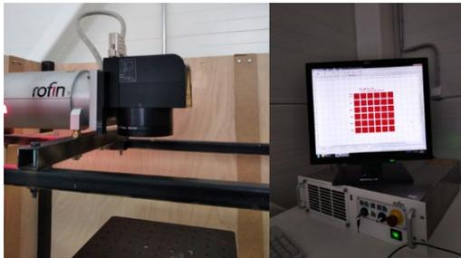
Fig. 1. Technological system with fiber laser Rofin PowerLine F20.
