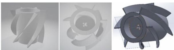
Fig. 4. Impeller with turned wings.
