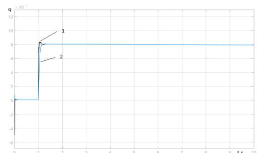
Fig. 16.b. Flow rate at the inlet (1) and outlet (2) of a 1 m pneumatic line.
