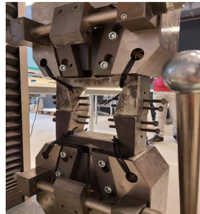
Fig.5. Tensile strength machine setup.
