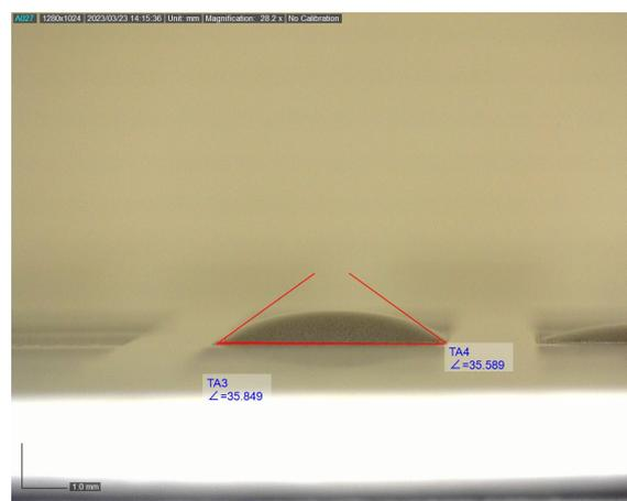
Fig.4.The measurement of the contact angle.
