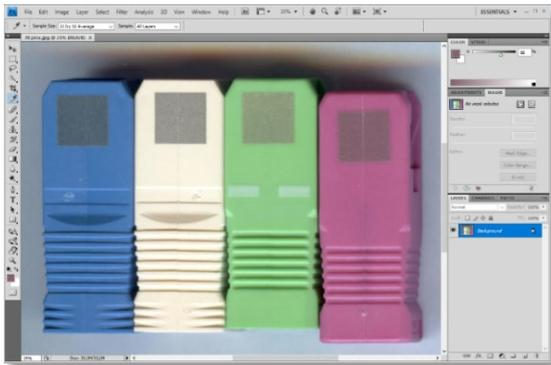
Fig. 1. Determining the value of the contrast marking on collar connectors using Photoshop.
