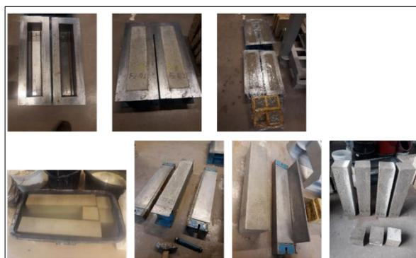
Fig. 5. The process of production of reinforced concrete and titanium concrete beams.
