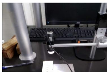
Fig. 3. Dino-Lite Edge AM7115MZT digital microscope.
