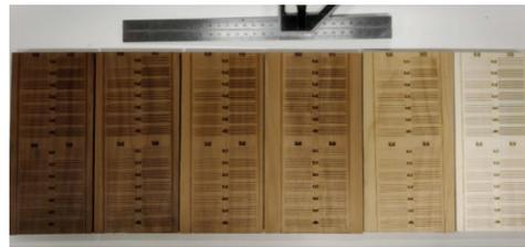
Fig. 5. Photograph of the six aspen wood samples engraved according to the created matrix, including five aspen thermowood samples and one natural aspen wood sample on the right.
