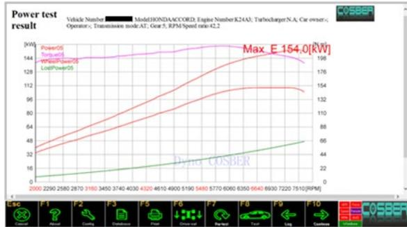
Fig. 6. Power performance of the passenger car and performance of the engine.
