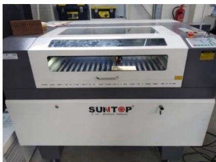
Fig. 2. CO<sub>2</sub> laser system SUNTOP ST-CC9060.
