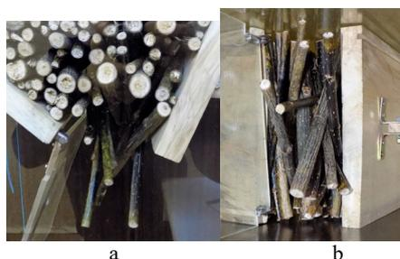
Fig. 5. Problems of unloading energy willow cuttings in the area of the unloading window.
