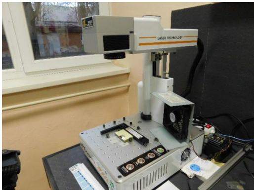
Fig. 1. Laser technological marking system.
