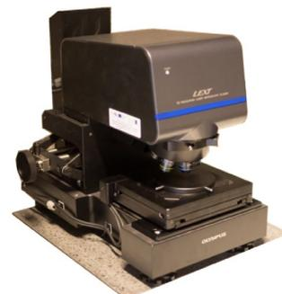
Fig. 2. Lext 3D measuring G Laser microscope OLS5000.
