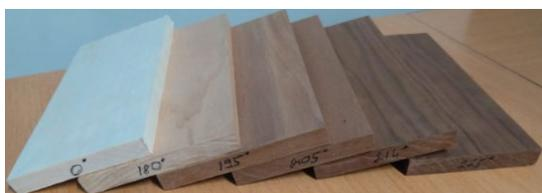
Fig. 1. Heat-treated aspen wood samples.
