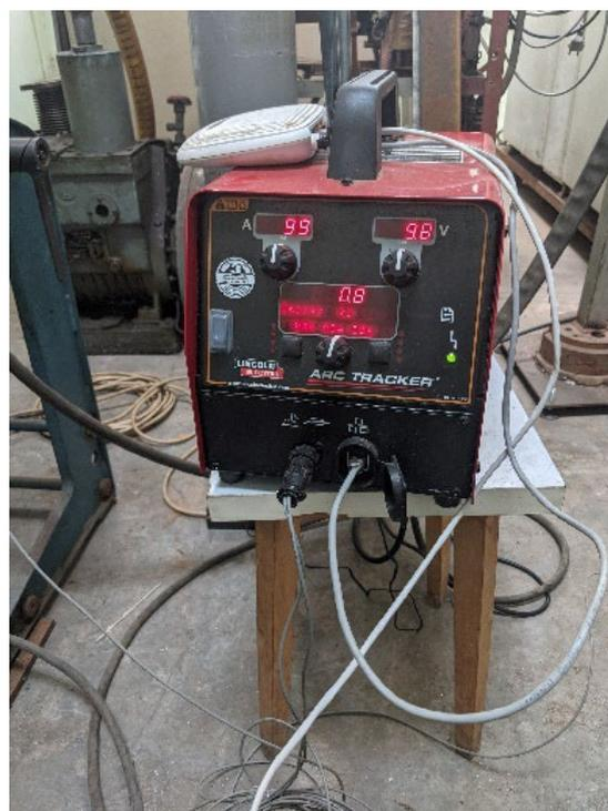
Fig. 6. Arc Tracker welding monitoring device.
