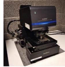
Fig. 2. Olympus LEXT OLS5000 3D Measuring Laser Microscope.
