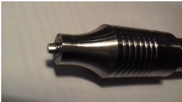
Fig. 1. Friction Stir Processing tool.
