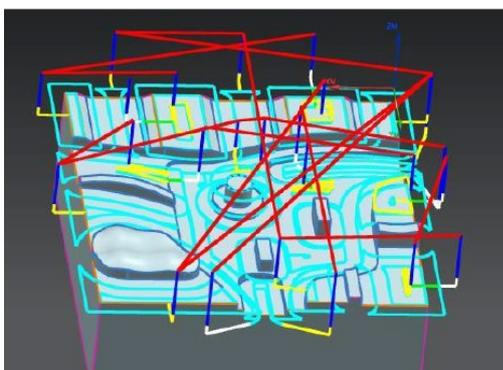
(a) flat face cylindrical cutter with  $D = 10$  mm.
