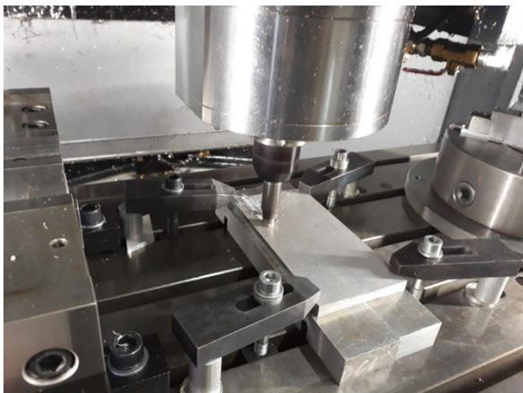
Fig. 2. Friction Stir Processing equipment.
