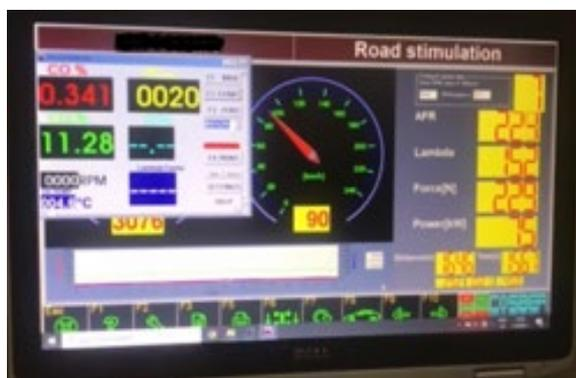
Fig. 6. Data from the software of Dyno Cosber 4000 and the gas analyzer, used in the experimental study.
