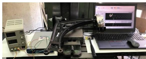
Fig. 7. Experimental determination of natural frequencies.
