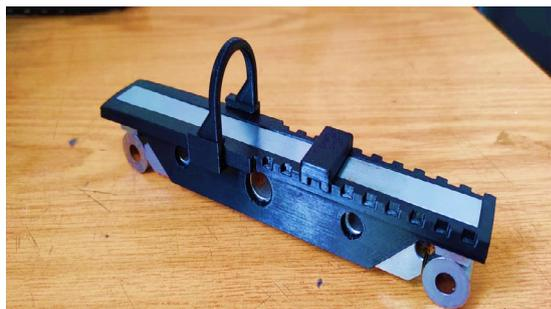
Fig.11 The device mounted on a 200mm sine bar.
