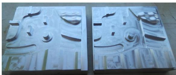
(a) detail 1 after finish milling by the variant without optimization
