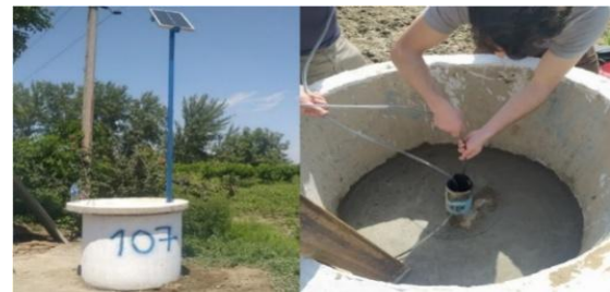
Fig. 3. The well equipped with a solar panel.
