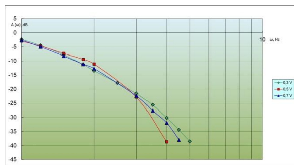
Fig. 6. AFR at input signal amplitudes of 0.3 V, 0.5 V, and 0.7 V
