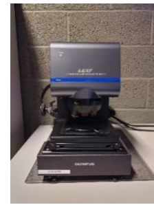
Fig. 2. Olympus LEXT OLS5000 3D Measuring Laser Microscope.
