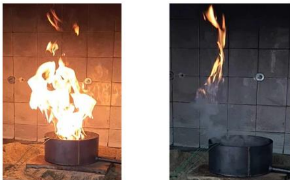
Fig. 2. Extinguishment due to the insufficient amount of fuel.
