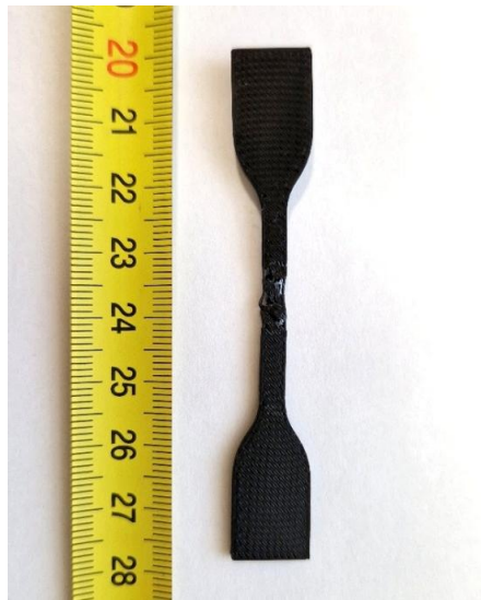
Fig. 4. Representative fractured tensile sample showing stress concentration in the centre region.
