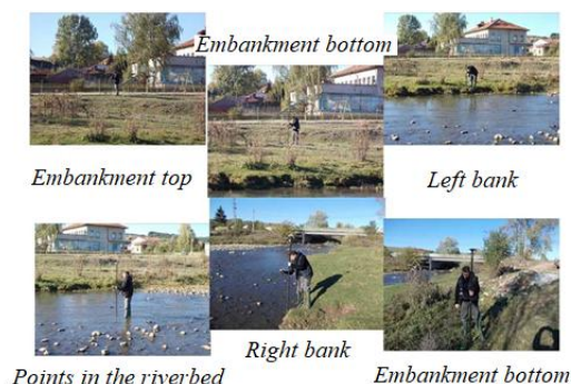
Fig. 6. Example of location of points for measuring a river profile [4]
