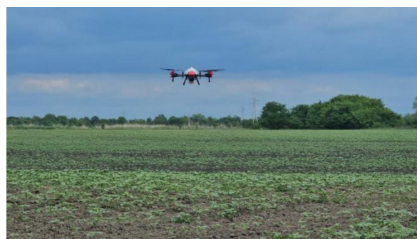
Fig. 3. XAG P40 drone when spraying sunflower.
