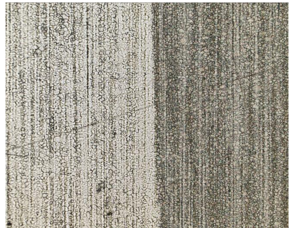
Fig. 9. Comparison of laser “polished” (left) and untreated surface (right).
