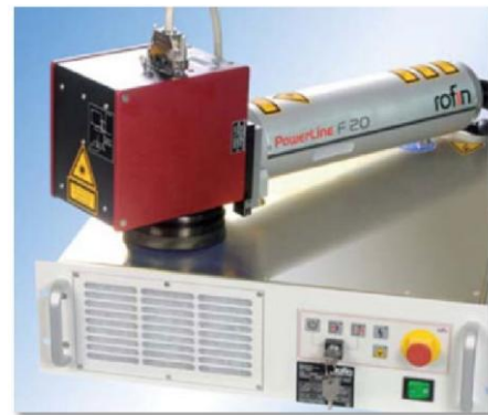
Fig. 1. ROFIN 20 W fibre laser system at Laser Institute of Rezekne Academy of Technology.
