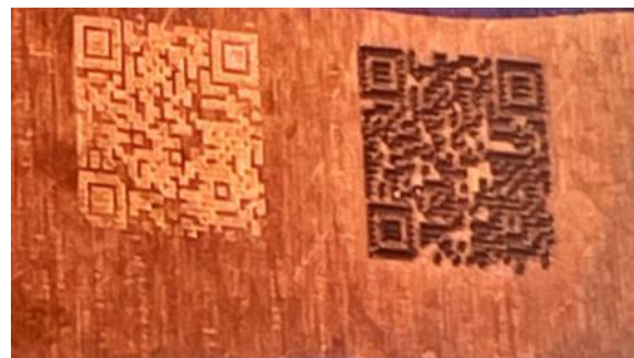
Fig. 8. Obtained QR codes on copper surface – starting from left end, white (light) and dark marking, respectively.
