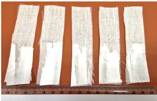
Fig. 4. Specimens from group S3 after T-peel testing.
